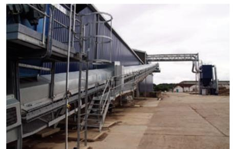
A giant conveyor belt will transport 80 000 tonnes per annum of plastics-rich automotive shredder residue to the ceiling of the plant.
