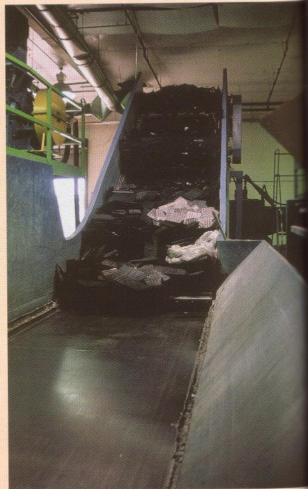
The emphasis at MBA Polymers is on automation. Here, unprocessed material makes its way up a conveyor toward the initial size-reduction stage.
