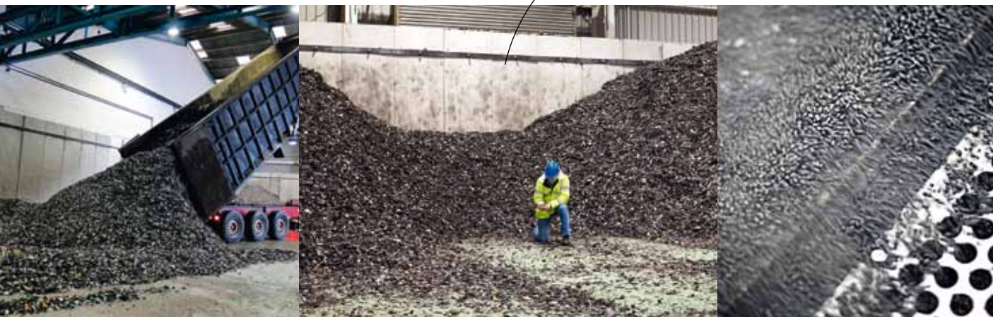
Mike Biddle examines "shredder residue" – the waste material from which MBA Polymers extracts pure high-grade plastic (below right)
