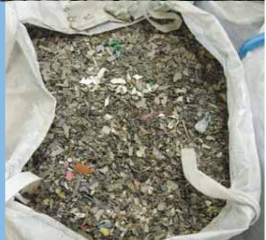
MBA Polymers has developed technology that can sort mixed engineering plastics (above) and produce virgin-quality recycled resin (top).
