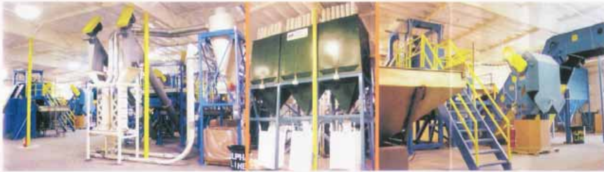
MBA Polymers' recycling plants cost between $14 million and $23 million to build—half the sum needed to construct a virgin plastic plant with the same output. To begin the recycling process, chunks of fax machines and computers are fed into hoppers and go through a series of automated steps—many borrowed from other industries—that suck out metal, wood, foil, dust, foam and the like.
